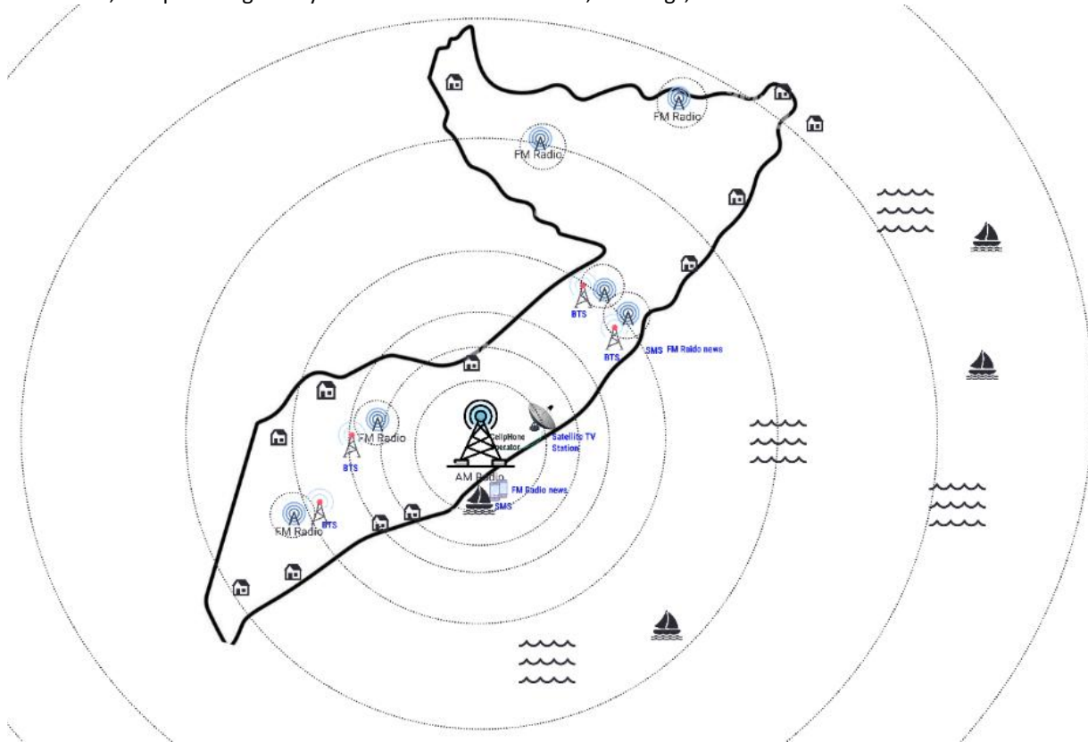
Figure 26 : Expansion of terrestrial broadcasts(AM Radio/TV) beyond the national boundary ( Source : Z M Sajjadul Islam )
