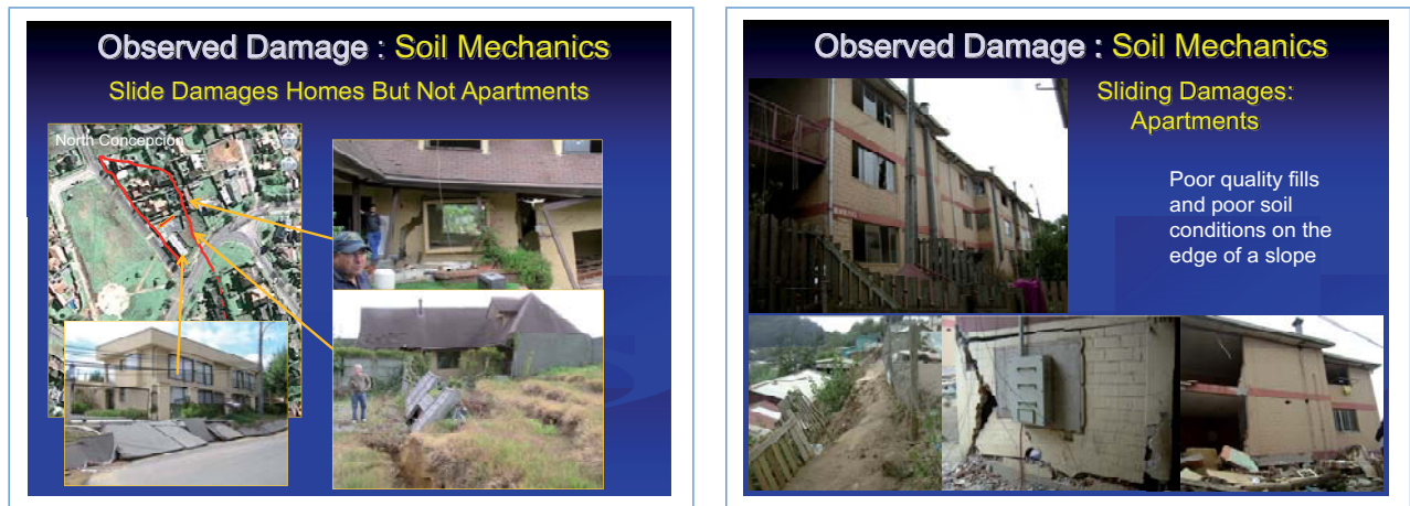
Figure 20 Failure of houses and small buildings due to landslides and poor soil conditions
